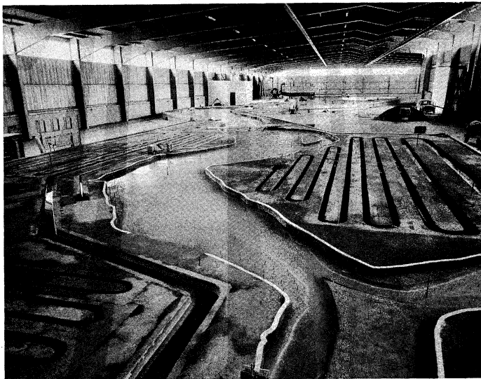
Figure 1: Tidal model of the Humber estuary in England.
